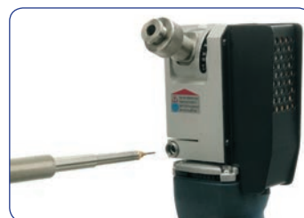
Precise adjustment of the stick-out
